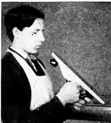
Fig. 11—Sighting the Bottom of the Plane
